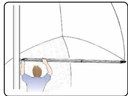
**1 Un-Cleat The Line    2 Pull Line To Extend The Pole    3 Re-Cleat The Line.**
