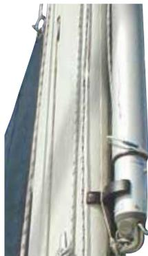
Storing poles (whisker or spinnaker) vertically up the forward face of the mast has become very popular. It clears the decks and keeps the cruising sailor from having to lift the entire weight of the pole from the deck to the mast car. By combining our VPC-125 T-Track Storage Chock with our fixed MPC Mast Chock with a running T-track system similar to the one shown to the right, you can create a highly effective vertical pole storage system.
